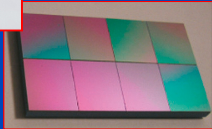
“Stellar detector”, modular and 2D tilable, focussed 1D anti scatter grid (Photo courtesy by Siemens)
