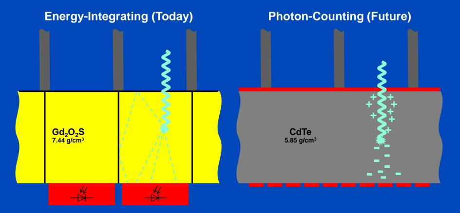
Requirements for CT: up to 10<sup>9</sup> x-ray photon counts per second per mm<sup>2</sup>. Hence, photon counting only achievable for direct converters.
