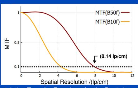
Modulation Transfer Functions for the Basis Images
