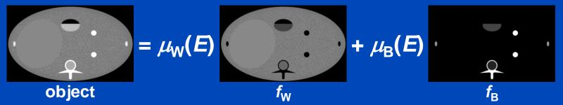
A measured ray consists of a spectrum w(E) and is attenuated by the object
