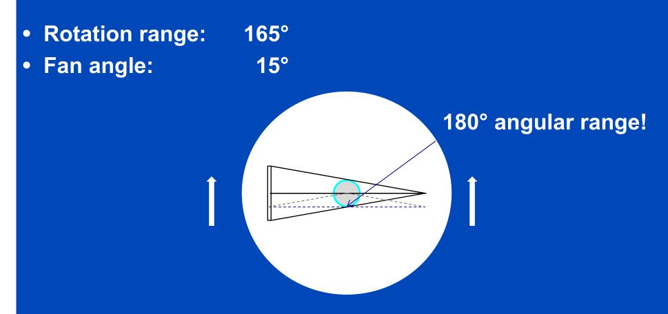
Rotate-plus-shift trajectory: Shifting the beam over the FOV increases the angular range by up to the fan angle  $\varphi$ .
