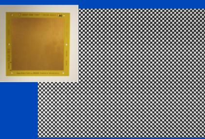
"Ideal" modulator (projection image of a copper modulator) Non-ideal modulator (projection image of the erbium modulator)
