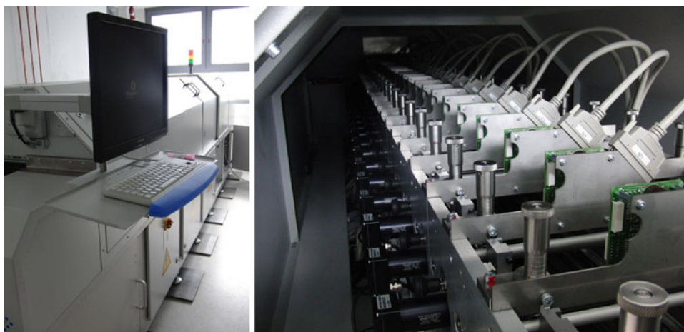
Fig. 2 Pictures of the latest laser printer generation: The 24 linearly aligned printing cartridges ( right ) in the printing track form the core of the 5.5 m long device ( left )
